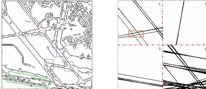
Fig. 2. (a): Edge map of a part of airport. Discontinuities of edges are due to intersections with taxi ways (blue boxes), to edge detector (red boxes) and to the nature of runways (green box); (b): Thresholded seed beamlets in the dyadic squares of  $128 \times 128$  pixel size.
