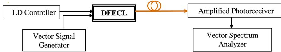
Figure 1 The setup for microwave transmission by DFECCL.
