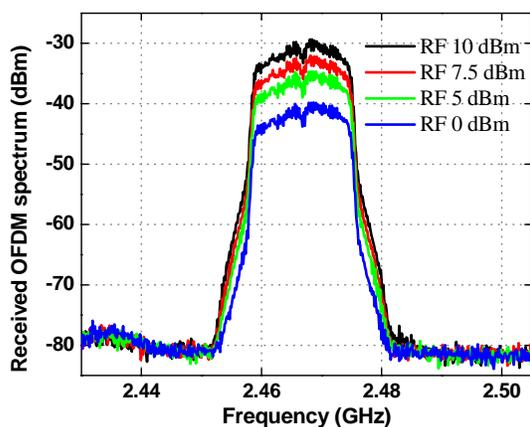
Figure 2 The received OFDM spectrum transmitted from directly modulating a DFECCL
