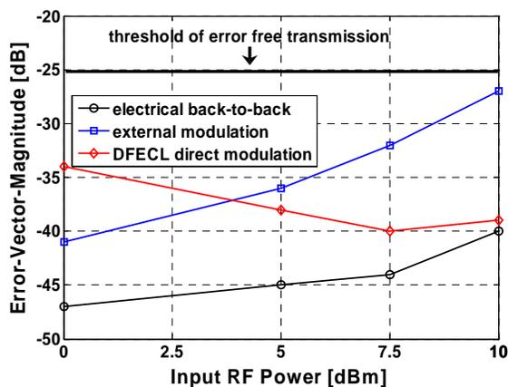
Figure 3 EVM measurement results versus different RF input power for the DFECCL and externally-modulated DFB laser diode.
