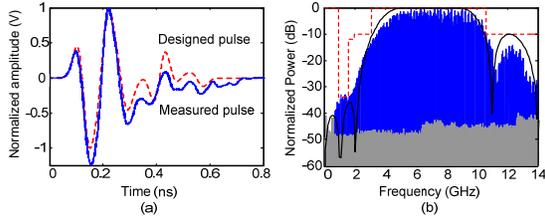
Fig.4. Measured UWB pulse (a) and the spectrum (b).
