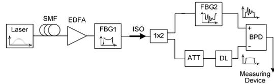
Fig. 2. Block diagram of the experimental setup.
