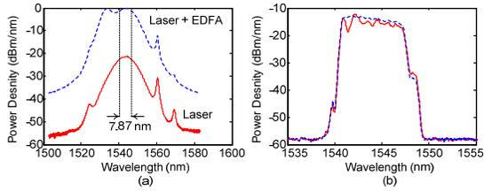
Fig.3. (a) Spectrum of the source before and after EDFA, (b) spectra in the two arms of the BPD.
