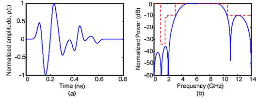
Fig. 1. Designed UWB pulse (a) and its spectrum (b).
