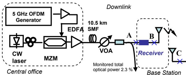
Fig. 1. Schematics of the ROF set-up.
