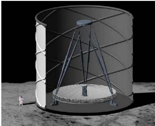
Artist's impression of the 20 m telescope. The secondary mirror is erected by extending the six telescoping legs and the sunshield by inflation. The scientific instruments are below the bearing pier, shielded by lunar soil. (drawn by Tom Connors).
