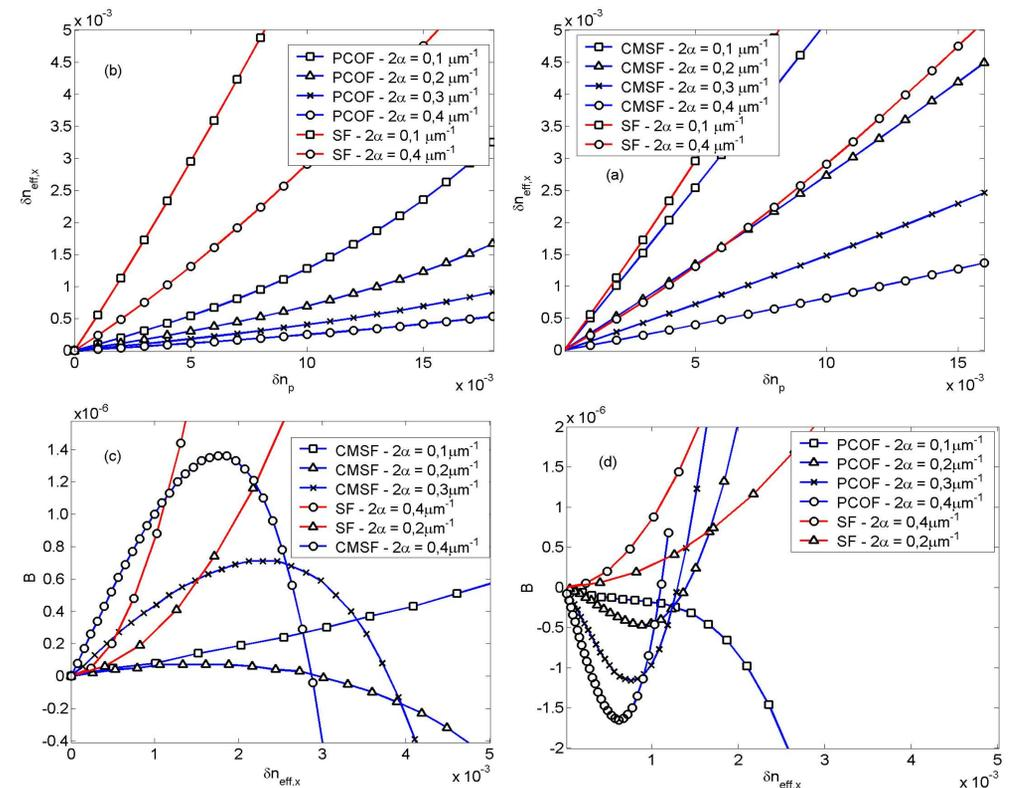
The effective index change (a-b) and the form birefringence ( $B = n_{eff,x} - n_{eff,y}$ ) (c-d) as a function of the peak refractive index change for CMSF and SF (a-c) and PCOF and SF (b-d).
