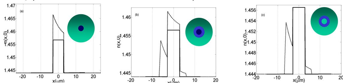
The transverse refractive index profile for (a) ST, (b) CMSF and (c) PCOF
